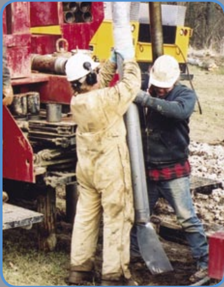
■ Installing poly core bag over core barrel prior to core extraction.
