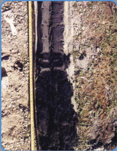
■ Continuous core sample showing interface between sand aquifer and confining clay layer.
